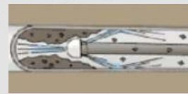
UNBLOCKED WITH HIGH PRESSURE JETTER
