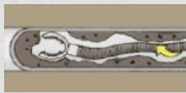
UNBLOCKED WITH A CABLE
